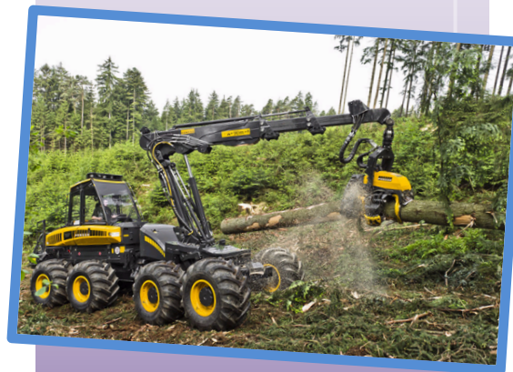
“Harvester” cutting trees to length
