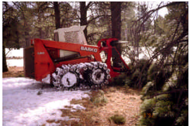
Photo 6 – “Micro” harvesting: cutting with a small shear
